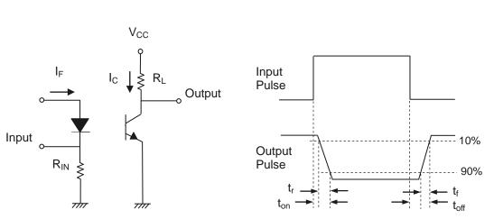
Figure 10. Switching Time Test Circuit & Waveforms
