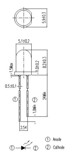
Note: Tolerances unless dimensions ±0.25mm
