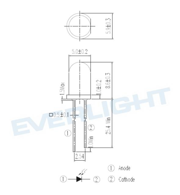
Note: Tolerances unless dimensions ±0.25mm
